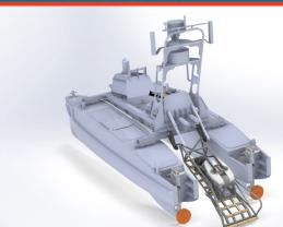
The robust, fully-welded marine-grade alloy construction is built under survey. REAV-60's principal dimensions enable the USV to be transported, launched and recovered by road-trailer, whilst its modular construction enables the system to be shipped inside a standard shipping container for rapid global mobilisation.
